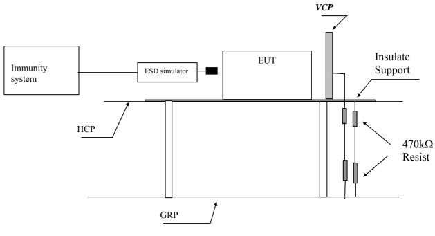
Note: HCP means <u>H</u>orizontal <u>C</u>oupling <u>P</u>lane, VCP means <u>V</u>ertical <u>C</u>oupling <u>P</u>lane GRP means <u>G</u>round <u>R</u>eference <u>P</u>lane
