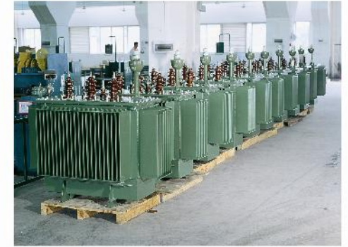
三相油浸式配电变压器生产线 Three phase oil immersed distribution transformer product line
