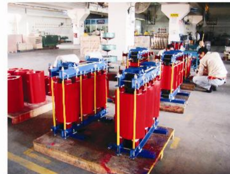
电抗器生产线 Reactor product line
