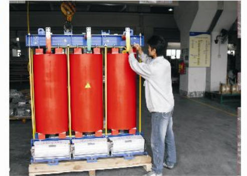
干式变压器生产线 Dry-type transformer product line
