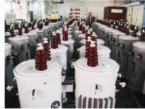
单相柱上式配电变压器生产线 Single phase pole mounted distribution transformer product line
